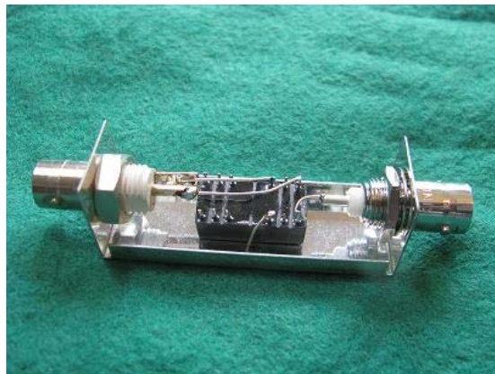
Fig 1 – A recovered filter assembled in a small tin-plate enclosure, with insulated output connector
